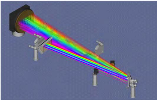
Figure 1: A 3D model of an optical stretcher designed with LaserCAD and rendered with FreeCAD.
