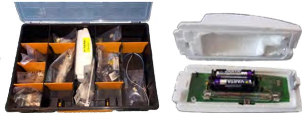
Figure 1: Soldering kit (left) and finished GMC (right).
