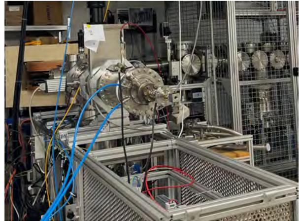
Figure 2: The sputter ion source mounted on the beamline. The electronics and power supplies reside in a high voltage cage below the ion source. The cooling of the target and the flange is realised from ground potential by a dedicated dielectric fluid.
