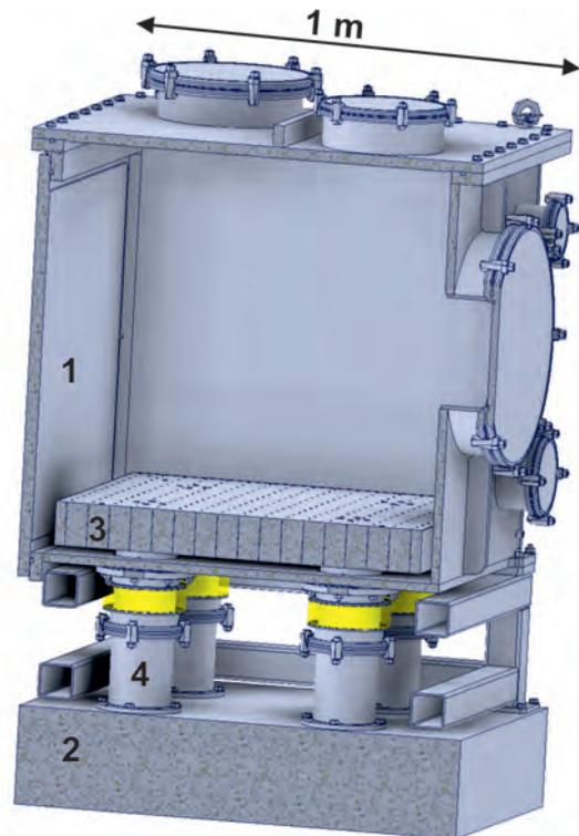
Figure 2: Sectional view of the wedding chamber. 1: vacuum chamber (1.0 m x 1.0 m x 1.4 m). 2: granite base (0.9 m x 1.0 m x 0.2 m). 3: breadboard. 4: connecting foot.
