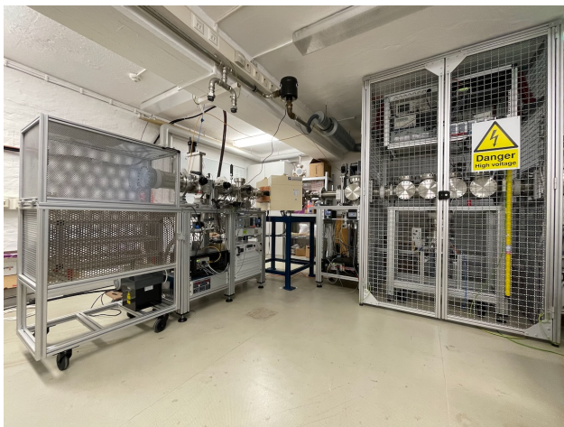
Figure 1: The LISEL setup at the University of Jena. On the left the ion source cage with the extraction lens. In the middle the double focusing sector field magnet. On the right the LISEL cooler inside the high voltage cage.
