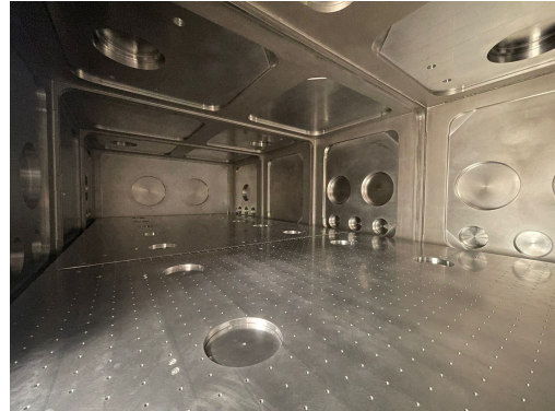
Figure 2: Interior view of the TAF target chamber. The holes in the breadboard are the heavy duty ports (see text).
