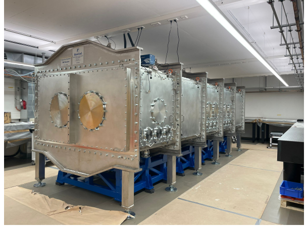
Figure 1: Exterior view of the TAF target chamber. The two ISO 500 flanges on the front are the connection ports for the TOR chamber.
