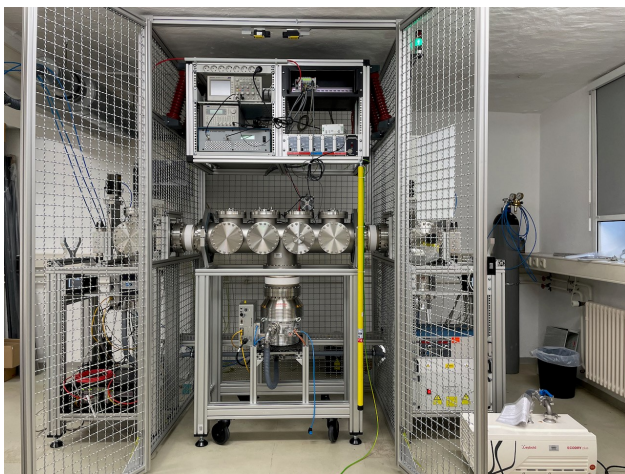
Figure 1: LISEL cooler setup with high voltage cage.
