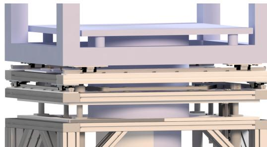
Figure 2: Stepper-motor-driven XYZ positioning unit for use with Blufors cryostat.
