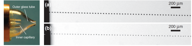
Figure 1: Left: Inner capillary for liquid jet generation and outer capillary for ambient gas allocation to prevent jet freezing. Right: Images of periodic droplet streams of a) argon and b) hydrogen [5]
