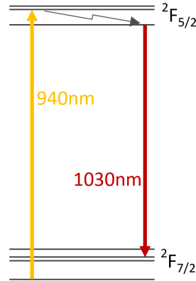
Figure 5: \text{Yb}^{3+} energy level diagram with typically employed manifolds.
