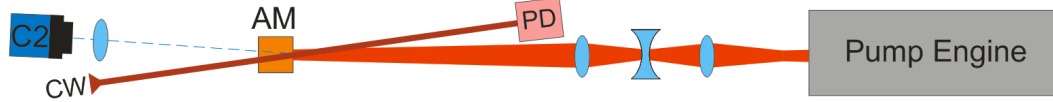
Figure 29: Illustrated setup of the gain measurement configuration. The pump laser passes from the pump engine, into a zoom lens setup, and onto the active material (AM). The measurement beam (CW - continuous wave) passes through the pumped active material and into a Thorlabs DET36A/M photodetector (PD) connected to an oscilloscope, which measures the signal strength throughout the pump cycle. A camera (C2) is used to image the plane of the pumped active material, in order to ensure proper CW/pump overlap and to capture the spatial fluorescence profile.
