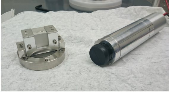
(a) Detector head and photomultiplier tube with aluminium casing.
