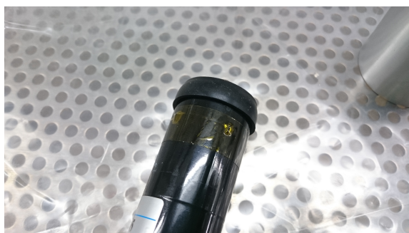
(a) Damage to the PMT from the aluminium casing.
