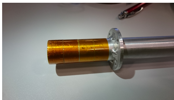
(b) Fixation rod isolated with kapton foil to prevent short circuits.
